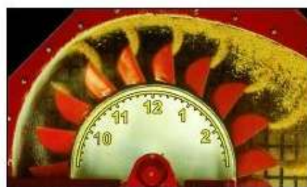
he al Test Elevator Fitted with Starco Elevator Buckets Showing Initial Discharge at 10 o'clock
