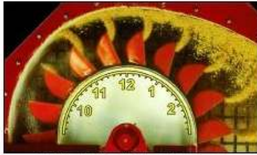
he al Test Elevator Fitted with Staroo Elevator Buckets Showing Initial Discharge at 10 o'clock
