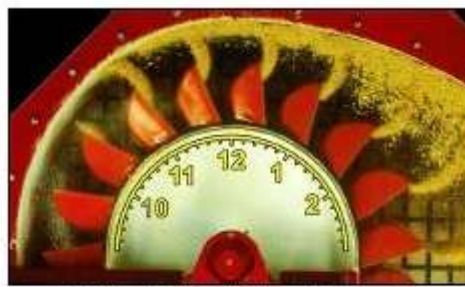
Test Elevator Fitted with Staro Elevator Buckets Showing Initial Discharge at 10 o'clock
